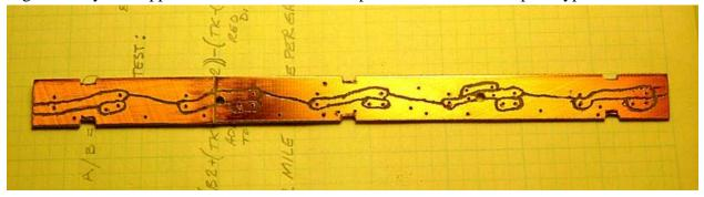
I added bright red LEDs in pairs with a dropping resistor for each pair.
