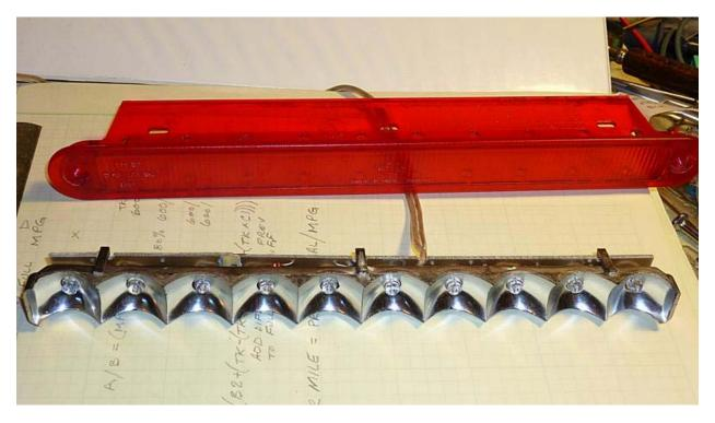
Here is the circuit board in place with the reflector ready to go back into the housing. The result was a success.
